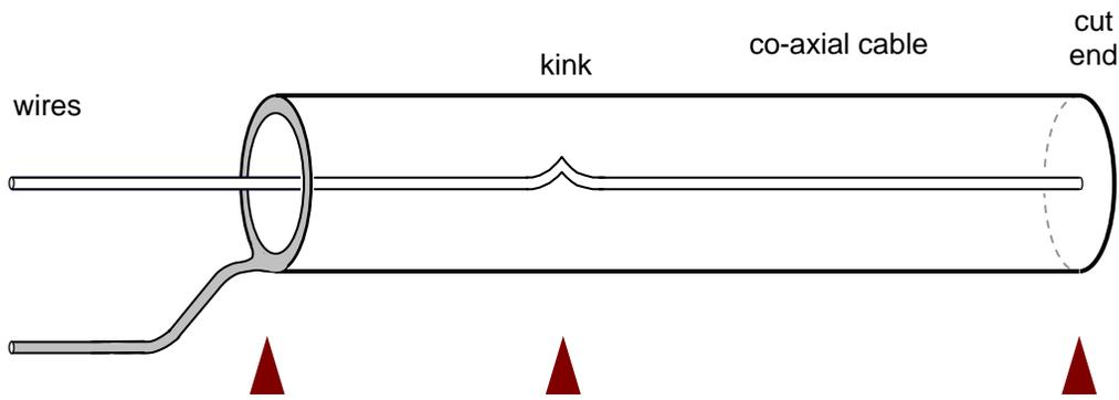
Fig C6-7/2. Examples of non-uniform wave-guides.
