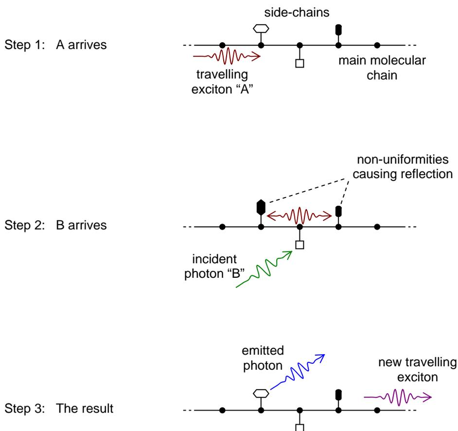
Fig C6.7/3. One possible molecular embodiment of an *and*-gate, with the following logical properties:- .....
