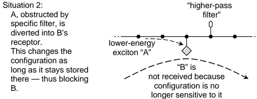
Fig C6.7/6. One possible molecular embodiment of “B and not A”, with the logical properties:-
