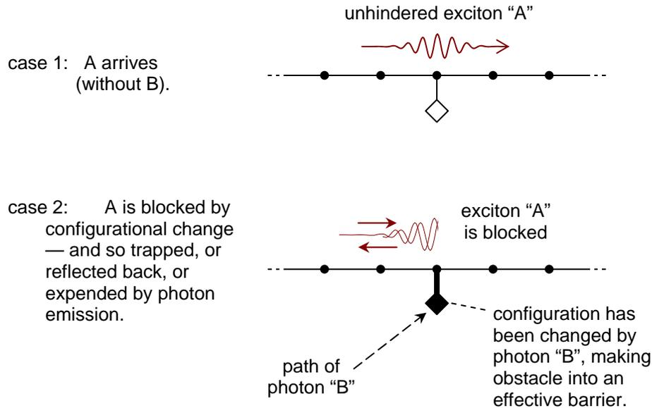
Fig C6.7/5. One possible molecular embodiment of “A and not B”, i.e. the logical condition depicted by:-
